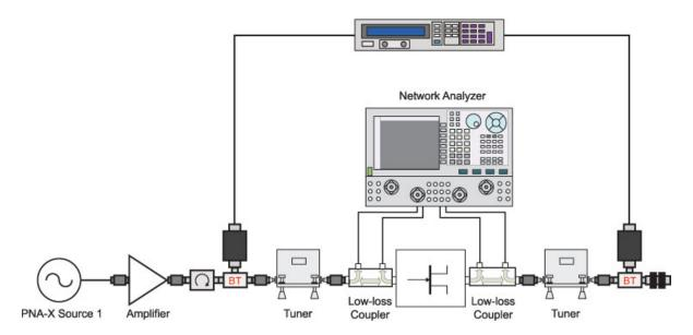
Some modern VNAs are capable of Nonlinear-VNA measurements (NVNA) including time-domain voltage and current waveforms and load lines, which can be useful for studying classes of operation. Vector-receiver load pull can be easily extended to NVNA-based load pull (as long as the VNA can perform NVNA measurements, so can the load pull system).
